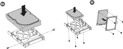
6-5. Insert the tray into the HDD Cage, and secure the SSD tray back onto the case with the thumbscrew.
